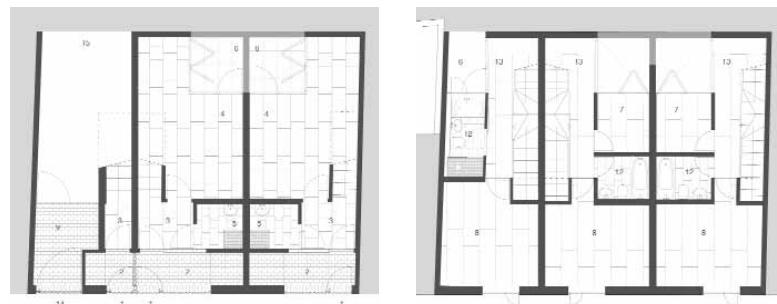
Three new houses on a small brown-field site: redevelopment at Chance Street, London [...] at Chance Street, London, ground and first floors
