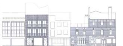
Above Aerial and east-facing elevation of the townhouse on Charlotte Road (gh: DG). Below Charlotte Road elevation; E-W section, two S-N sections: 1 retail, 2 wc, 3 residential entrance, 4 living room, 5 void, 6 bedroom, 7 utility, 8 living room, 9 terrace, 10 bathroom, 11 first floor landing, 12 courtyard
